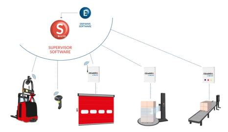
The management system takes the dimensions of the robots, creates the route by using the information provided by the Balyo installer (i.e., prohibited parking zones, pedestrian crossings, fire doors, etc.) and optimizes vehicle traffic in real time thanks to an algorithm developed by the Company in order to avoid bottlenecks and collisions between robots.
